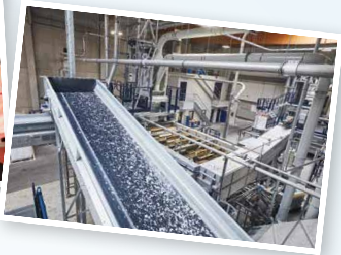
A multi-stage process is used to separate the plastics from the shredded fridges according to type
