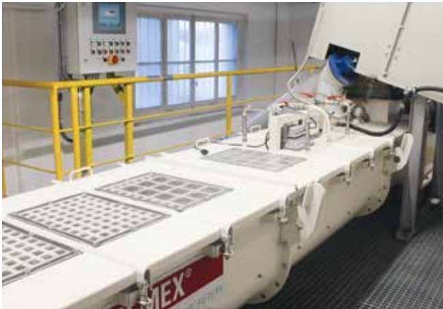
The new facility binds asbestos in concrete blocks that can be placed cleanly into – and retrieved from – a landfill's storage area
