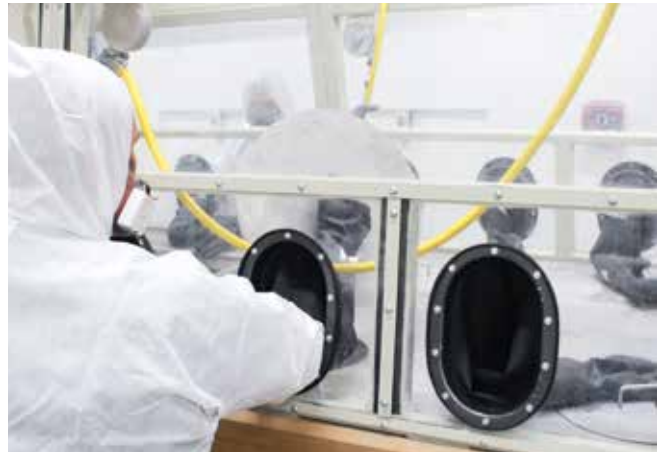
Operatives must wear personal protective equipment and may only handle the material using gloves attached to glove ports
