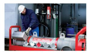
Damaged high pressure steel cylinders are normally no longer able to be transported; but this is no problem for us. We have special salvage packaging to transport them in.
